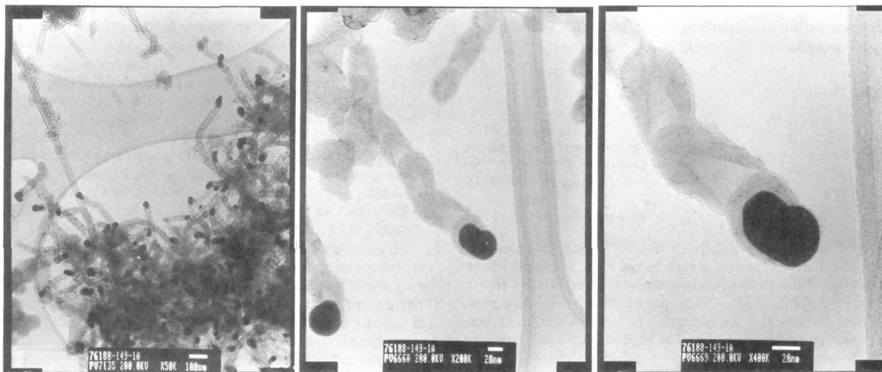
Figure 1. Electron micrographs of the core of the cathode deposits, showing many wormlike nanostructures with carbon-encapsulated palladium heads. (a, left) A magnification ratio of 125 000, (b, middle) a magnification ratio of 500 000, and (c, right) a magnification ratio of 1 000 000 showing the palladium head. Although the carbon shell looks amorphous in the micrographs, the electron diffraction and X-ray data show that it has the same lattice constants as the carbon nanotube and polyhedra. It is possible that the shell has some defects or is covered by other carbon which obscures the lattice image.
